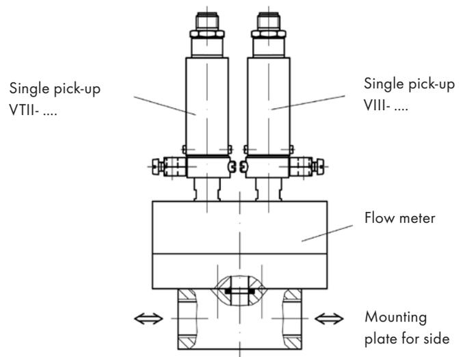
Figure 3: Application with directional detection
