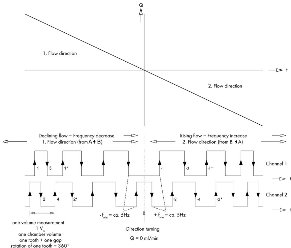
Figure 4: Signal output with two single pick-ups
