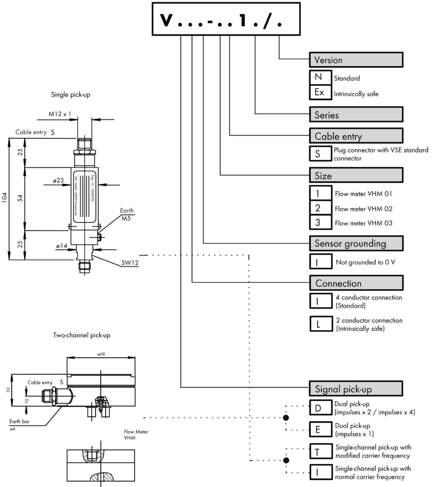
\* With the VDB series... (fiber-optic output), the signal can only be doubled (pulse x 2)
