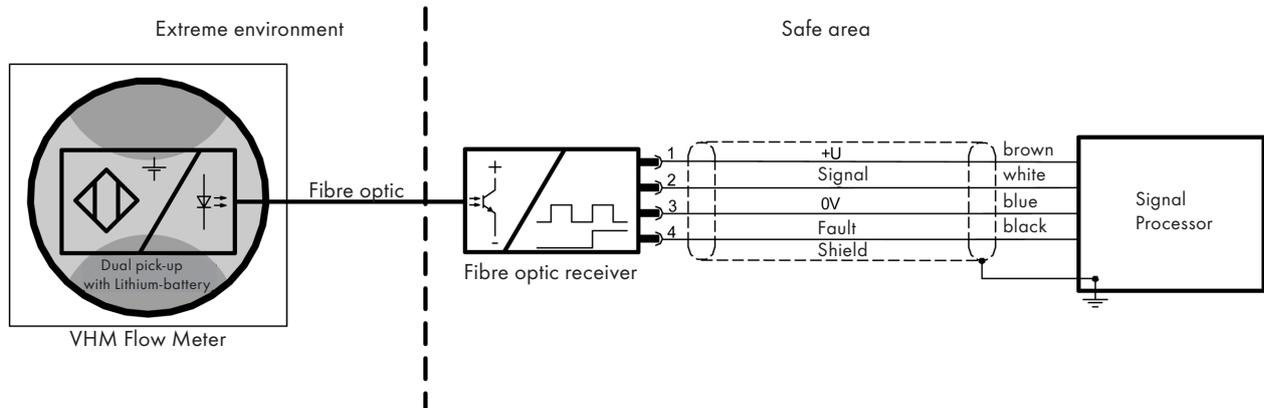
Figure 3: Wiring diagram for the measuring system
