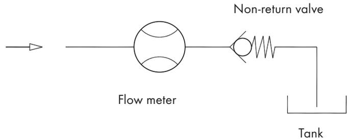
Figure 1: Flow meter with backpressure
